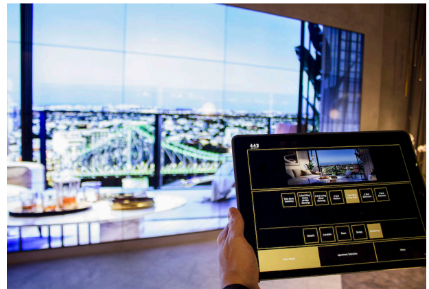
10k resolution video wall controlled by Present Plate app on iPad
